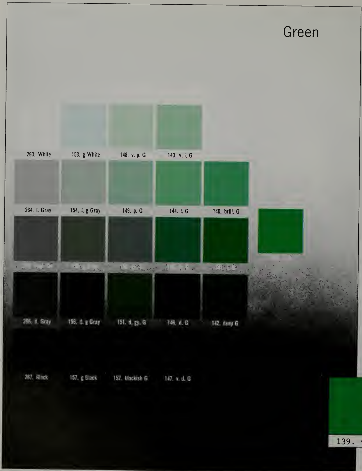
FIGURE 10. A photograph of the Green ISCC-NBS Centroid Color Chart. A single color sample with its Centroid number and equivalent ISCC-NBS color-name abbreviation is shown in the small insert.
